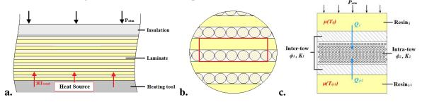
**Figure 1:** Physical representation of the model; (a) a thick laminate (40 mm) has heat applied from the bottom surface and is insulated on the top surface, (b) the laminate is made up of 'semi-preg' plies, which can be viewed as unit cells, (c) the unit cell in the model can account for flow from both its own resin layer and the resin layer below.
