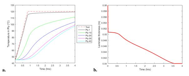
Figure 2: Results of the resin flow and heat transfer model; (a) significant thermal lag in the plies further from the tool surface, (b) laminate thickness reduction slows as the resin begins impregnating the tows. The heating rate was 1.5 C/min until the tool surface temperature reached 120°C and then it was held constant
